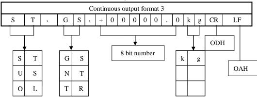
Header1 Header2 Header 1 ST(Stable) (Unsable) US (Over Load) OL Header 2 GS (Gross data) NT (Net data) (Tare data) TR
